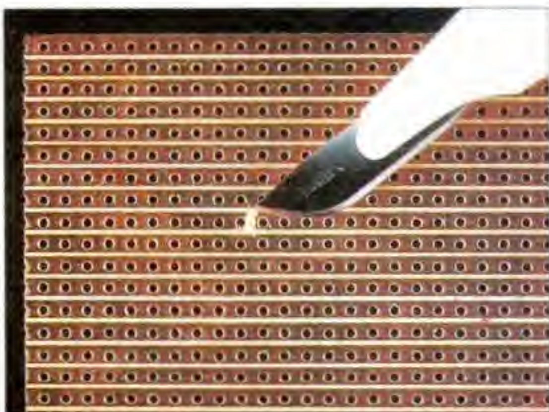
To break unwanted connections, cut at both sides with a sharp knife and peel off the conductive material.
